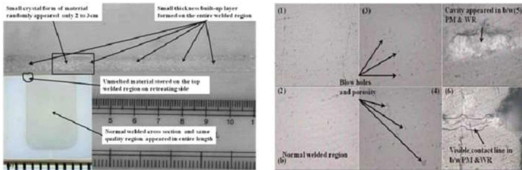
**Figure 6: a & b Appearance and Microstructure of FSW Region for Square Pin at 1200 r/min and 40 mm/min**
