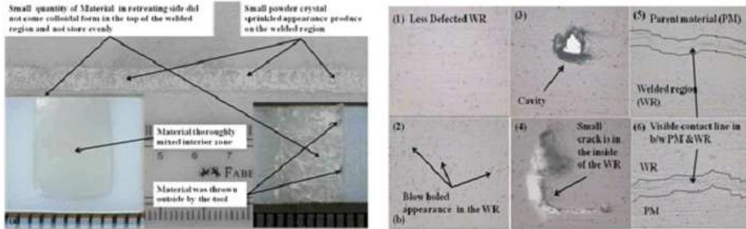
Figure 3: a & b Appearance and Microstructure of FSW Region for Square Pin at 600 r/min and 10 mm/min
