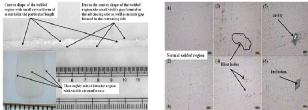
**Figure 11: a & b Appearance & Microstructure of FSW Region for Threaded Pin at 1000 r/min and 10 mm/min**
