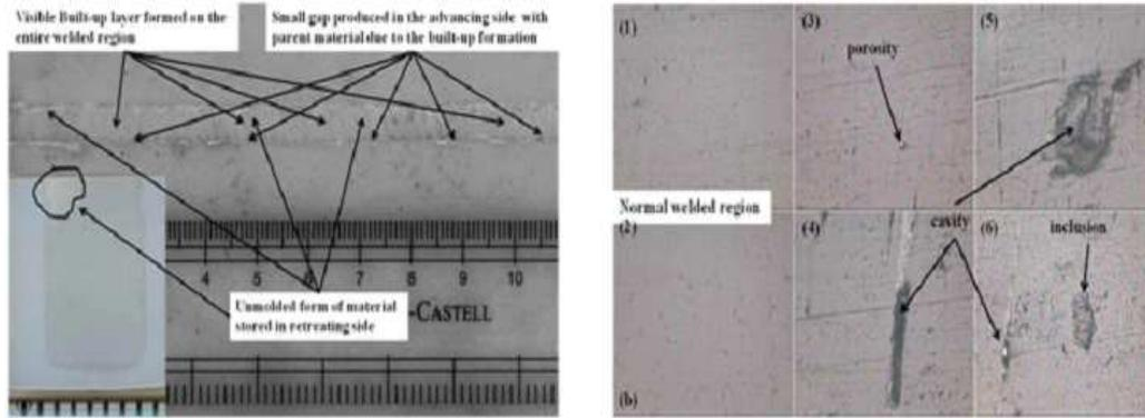
**Figure 10: a & b Appearance & Microstructure of FSW Region for Grooved pin at 1000 r/min and 40 mm/min**
