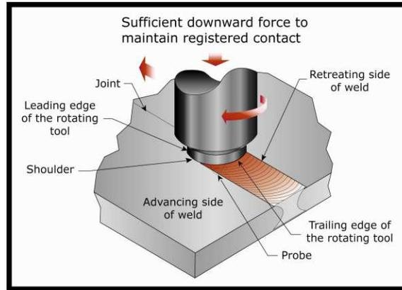
**Figure 1: Friction Stir Welding Process**
