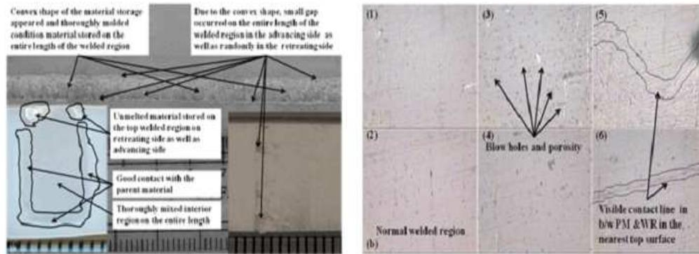
**Figure 8: a & b Appearance and Microstructure of FSW Region for Grooved Pin at 600 r/min and 20 mm/min**
