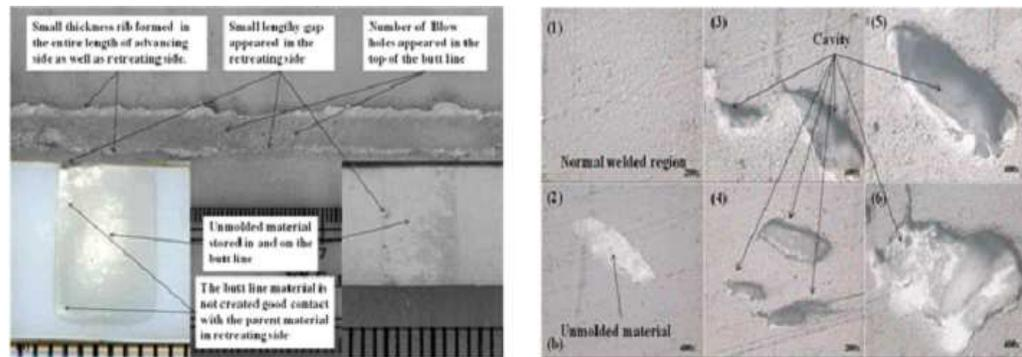
Figure 16: a & b Appearance & Microstructure of FSW Region for Triangular Pin at 1000 r/min and 20 mm/min
