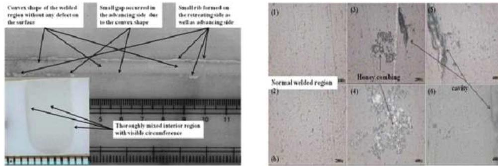
**Figure 12: a & b Appearance & Microstructure of FSW Region for Threaded Pin at 1200 r/min and 20 mm/min**
