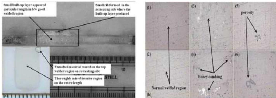
**Figure 7: a & b Appearance and Microstructure of FSW Region for Grooved Pin at 800 r/min and 10 mm/min**
