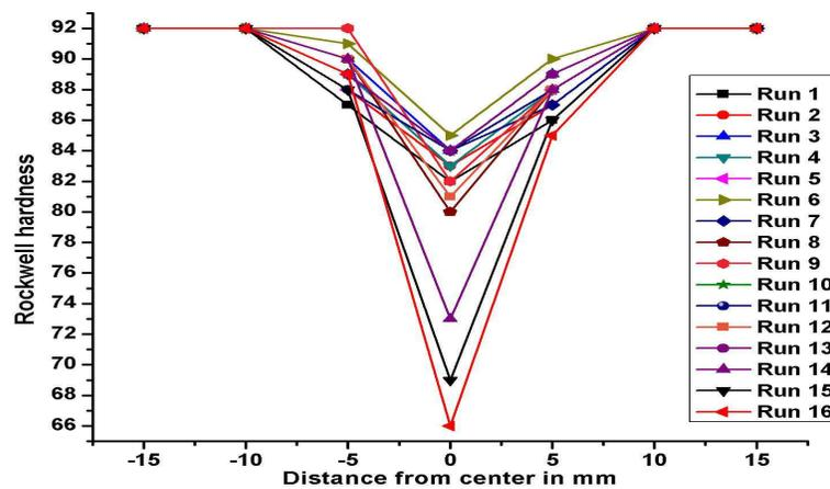
Figure 19: Effects of Different Process Parameters on Hardness
